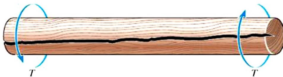
Failure of a wooden shaft due to torsion.
