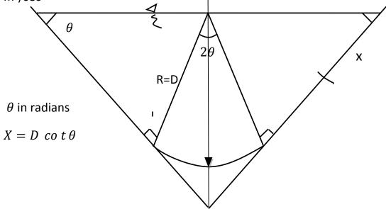
The radius of the bottom is equal to the depth of water (D). The angle in the center is  $(2 \theta)$
