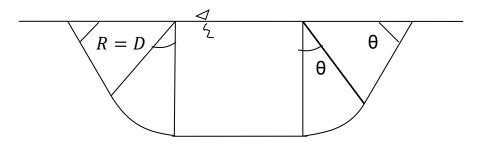
The trapezoidal section for the lined canals with discharge greater than 50  $\mbox{m}^3/\mbox{sec.}$
