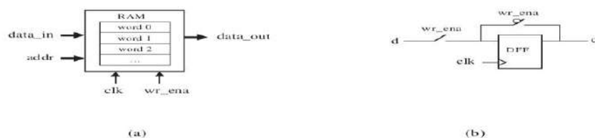
Figure 9.25 RAM with separate in/out data buses.
