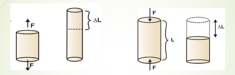
**Elongation:** The deformation that results from the application of tensile stress. An alloy with **high percent of elongation** can be bent or adjusted without danger **of fracture.**
