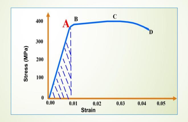
■ Toughness: It is the total work or energy required to break the material. It's the total area under the stress-strain curve. It requires strength and plasticity .
