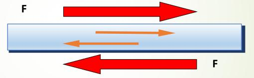
Shear force is the force which causes tearing a paper or a card. If one part of the crown is in occlusion while the rest is not, shear stress will develop.
