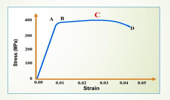
► Fracture Strength (point D): The stress at which a material fracture. The fracture strength is not necessarily the ultimate stress at which the material will fracture.
