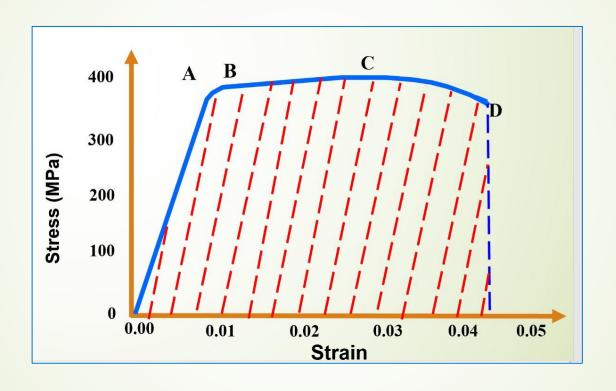
Properties of Stress-Strain Curves The shape of a stress-strain curve and the magnitude of stress and strain allow the classification of materials as regard to their properties e.g. weak, strong, flexible, stiff, ductile, brittle, resilient and tough.
