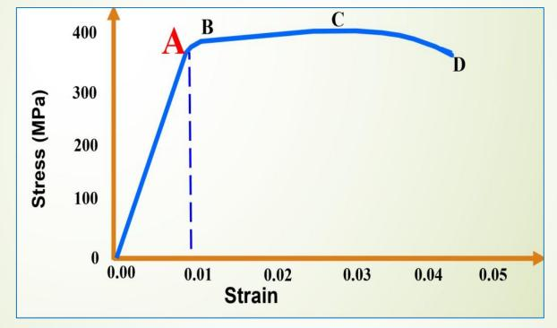
The region of the s-s curve before the proportional limit is called the "elastic region" (from 0 to A). • The region of the curve beyond this proportional limit is called as "plastic region" (from A to D).
