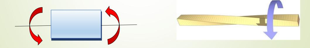
When external force or load is applied to a material the phenomena of strain occurs; i.e. the change in the dimensions of the material.
