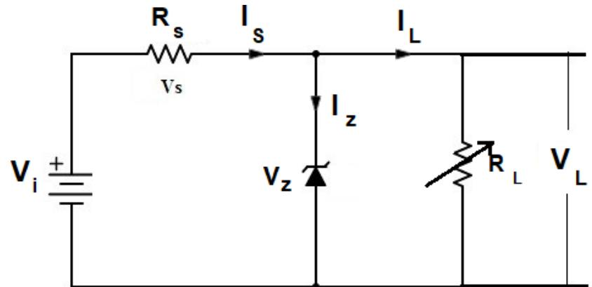
$$R_{Lmin} = \frac{V_z}{V_i - V_z} R_s$$
