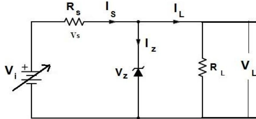
$$V_{i \min} = \frac{R_L + R_s}{R_L} V_Z$$
