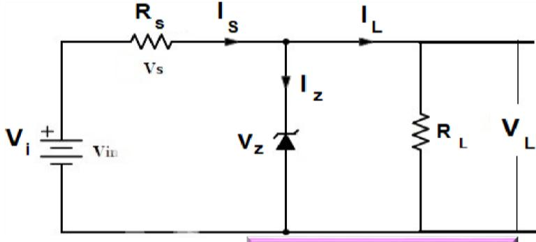
$$V_L = \frac{R_L}{R_L + R_s} V_i$$
