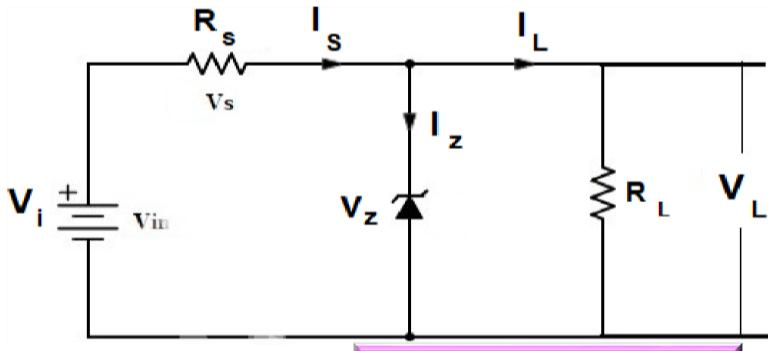
$$V_L = \frac{R_L}{R_L + R_S} V_i$$
