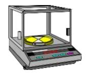
**Balances** are used to determine the mass of areagent or object.
