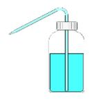
**Wash bottles** are used for dispensing small quantities of distilled water.
