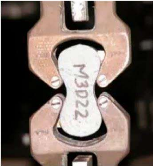
Figure 2.3-11: Samples of concrete direct tension specimen (3).
