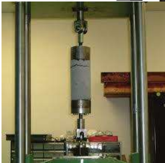
Figure 2.3-10: Samples of concrete direct tension specimen (2).
