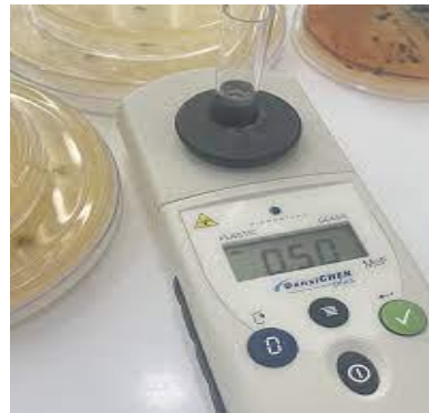
Figure (2) shows densichek attached with vitek device
