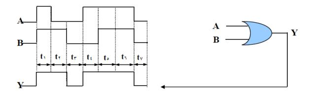
**Summary:** If inputs **A OR B** are high (or both) then the output is high. **Abbreviations:** often a '+' is used to signify the **OR** operator when writing Boolean equations.
